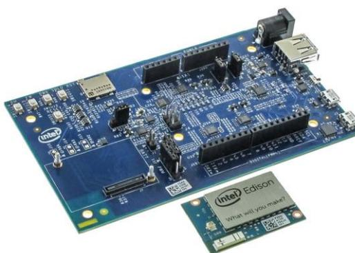
**Figura 6 – Intel Edison e Arduino da Intel**
